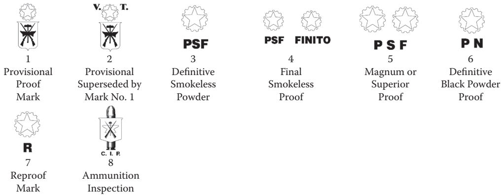
Figure 5.24 Italian proof marks. Note that the provisional mark represented by the crest of arms of Gardone Val Trompia. PSF means polvere senza fumo (smokeless powder). The bore diameter in gauge, caliber, or millimeters may be stamped. The barrel weight (expressed in kilograms) may also be present. A note about Italian proofing: If the firearm was proofed before 1954, Arabic numerals were used to indicate the date. From 1954, a code of Roman numerals was used. From 1975, the year is indicated by a two-digit date in a rectangle. (Source: BATFE Firearms Identification Guide.)
